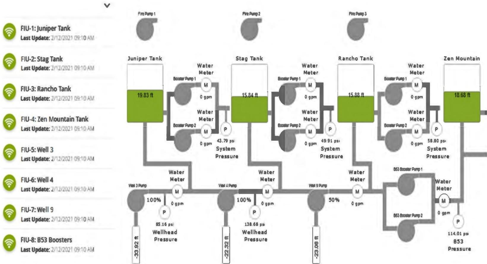
**Figure 3-19 Example Setup of SCADA System for LSCSD**
